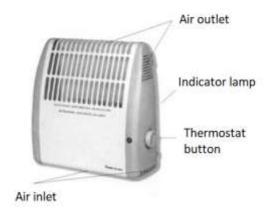
Turn the thermostat button until the indicator lamp will light up. This means the heater is heating. Turning the button back or forward, it will adjust on which temperature the thermostat will turn off or on.
